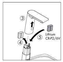
**Reset the faucet:** Remove the set screw with a 2.5 mm Allen wrench.
